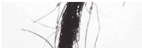
Open ended yarn provides low strength to fabric
